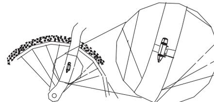
2. Screw the magnet onto the spoke.
